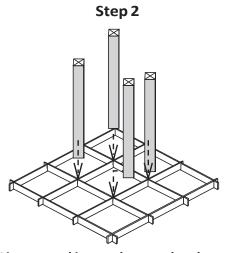
Line up and insert the wood rack pieces into the metal frame. Use a rubber mallet to install into the metal cross frame. Repeat until all wood rack pieces are installed.
