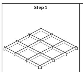
Assemble the bottom metal frame on a flat surface.
