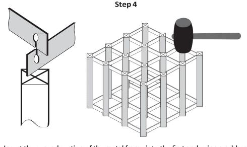
Insert the second section of the metal frame into the first and using a rubber mallet complete the installation into the wood pieces.
