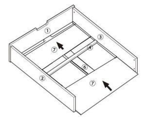
As the illustrated direction, slide the parts (Part 4 & 7) into the assembled parts in step 2.
