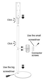
(2): Find the top of plate, insert it directly into the top of the aluminum tube while you hear the sound of click then installed;
