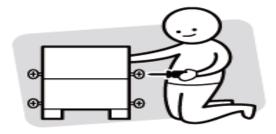
Do not fully tighten all screws until step/ precess finished.
