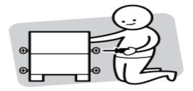
Do not fully tighten all screws until step/ precess finished.
