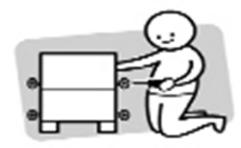
Do not fully tighten all screws until the step/process has been completed.
