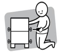
Do not fully tighten all screws until the step or process has finished.
