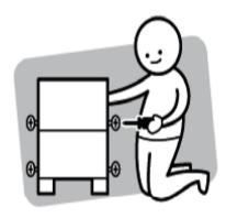
Do not fully tighten all screws until the step or process has finished.
