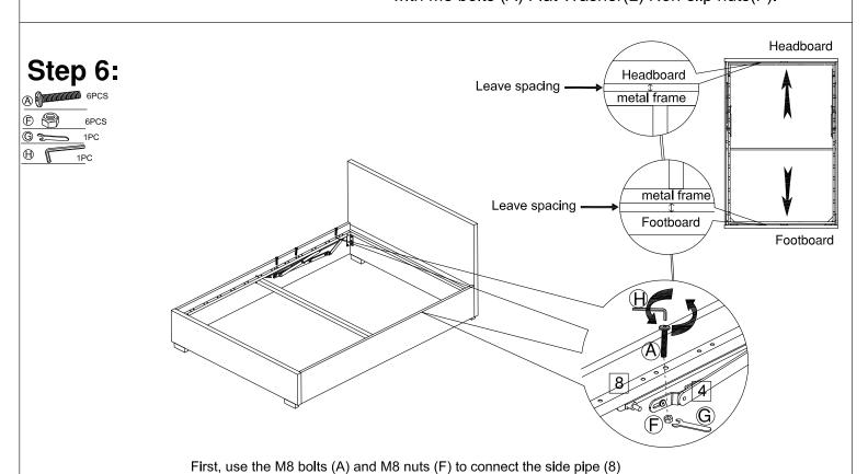
to the hinge (4). At this stage, do not fully tighten the M8 bolts (A) to allow for some adjustment between the headboard, footboard and metal frames. There should be some spacing between the headboard, footboard and the metal frames. Once every part is aligned, fully tighten all M8 bolts (A).
