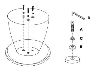
Lay the tabletop (1) on the ground with a screw hole upwards, followed by keeping the table frame (2) on the tabletop with a screw hole upwards. Then, properly install the flat washer (B), spring washer (C) and screw (A) in the screw hole and fasten it using the hex key (D); turn the table upright, and you are ready to use it.
